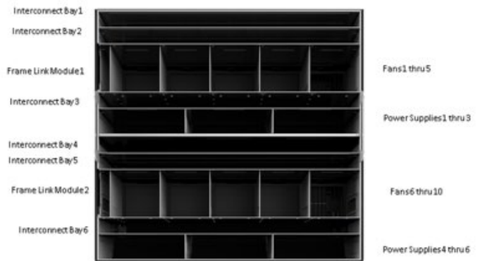
HPE Synergy 12000 Frame - Rear View
