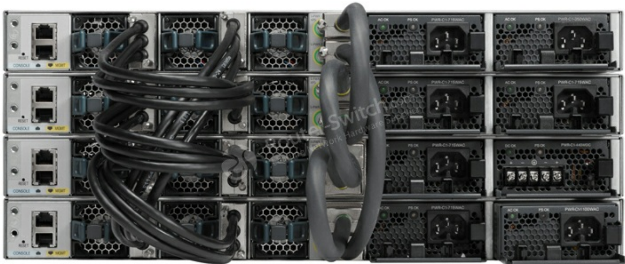
Figure 3 shows the StackWise-480 and StackPower connectors.
