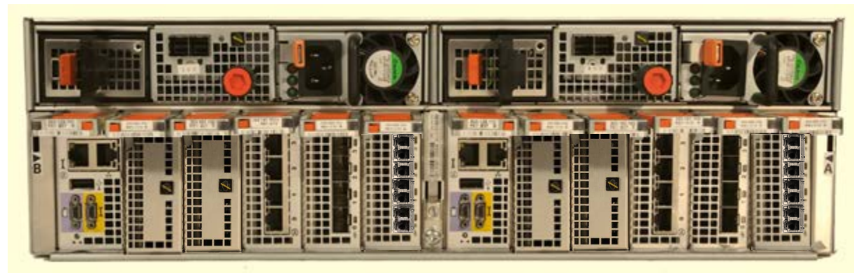
Figure 25. Back view of the DPE with SP A (on the right) and SP B (on the left)
