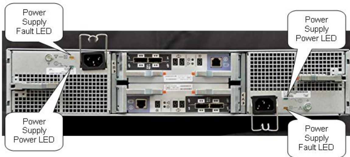
Figure 8. Back of the 25-drive DAE housing 2.5" drives
